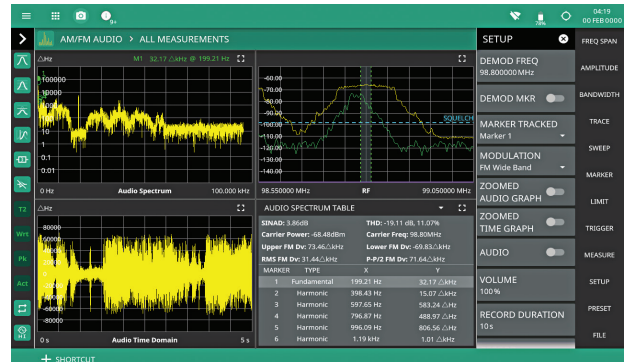
The AM/FM Modulation Measurements Screen Provides a Unique Simultaneous Display of Results and RF and Audio Spectrum
