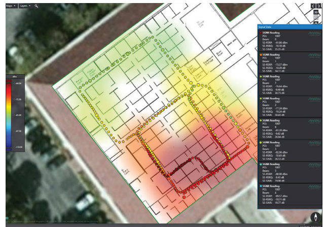
3D Indoor Maps with Base Station Data are Generated by the NEON Signal Mapper
