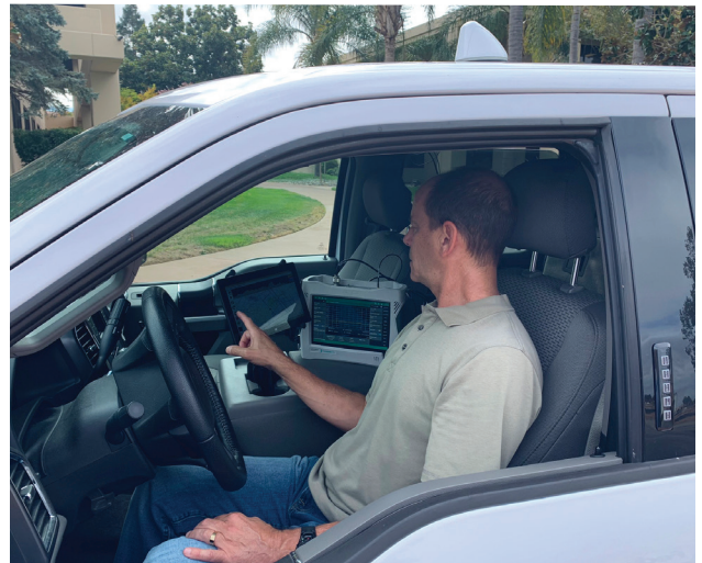
MIH System Installation with Large In-Vehicle Display and Omni Antenna on Roof
